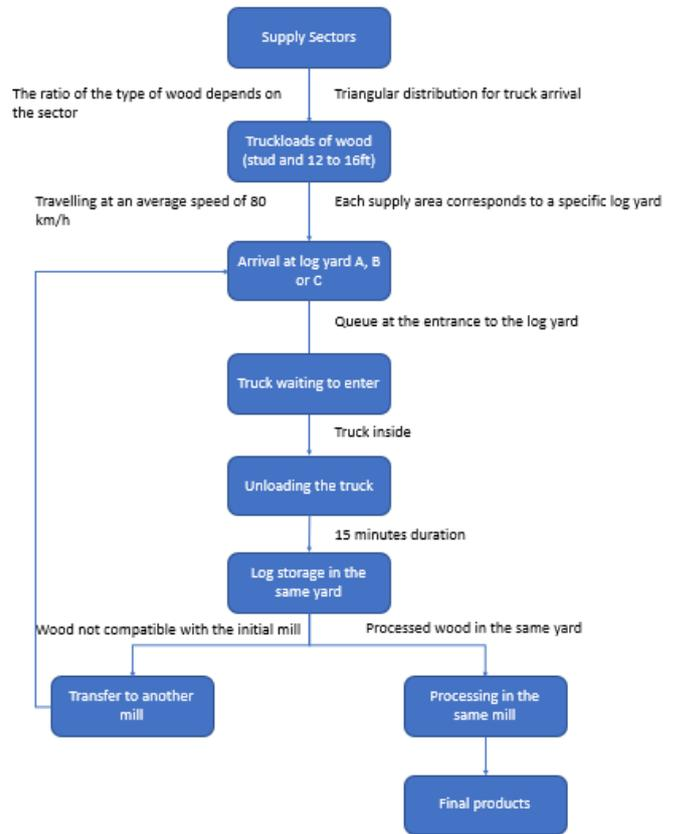
Figure 4. Simulation model operating process
