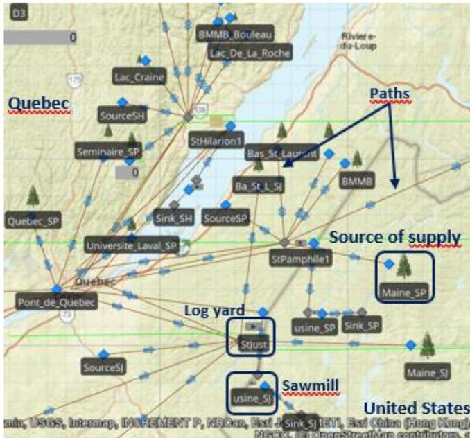
Figure 3. Simulation model components
